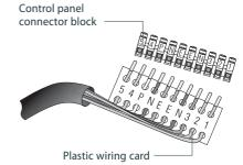
Fig. 3 Using the plastic wiring card to align the numbers/letters on the harness with those on the control panel connector block.
